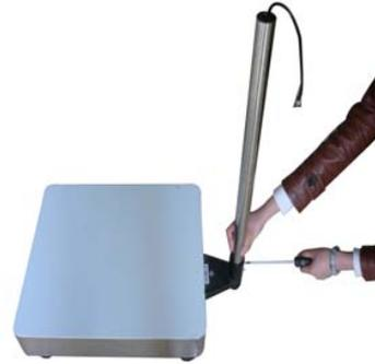
Step 2: After threading the Load Cell wire Through the bracket (3), attach the bracket to the Upright pole and then lock it with the screw (6).
